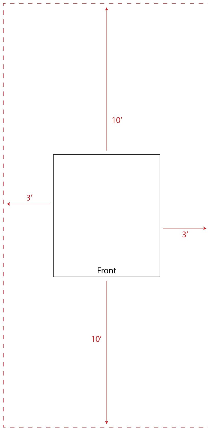
10 feet of clearance required for front and back of panel.
