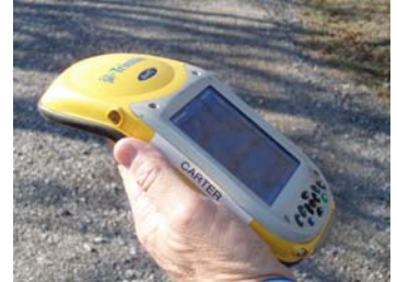
This hand held recorder gives Cooperative employees the ability to precisely locate the position of the power pole and inventory the distribution facilities it supports.
